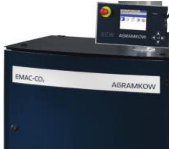
**EMAC CO<sub>2</sub>:** Cool Point planned to shift to Environmental friendly Refrigerant for their chest type bottle coolers for this they turned to CO<sub>2</sub> (R744). According to its chemical Properties, it makes the unit Eco Friendly and project is driven by a multinational company.
