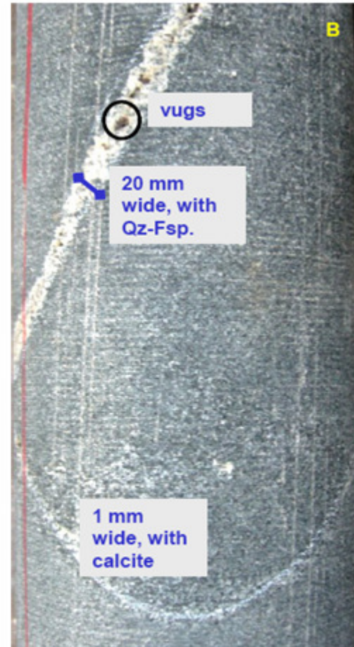
B: Photo of Core piece # 25 @ 2477.7 m (2481.7 m). The quartz-feldspar vein of about 20 mm wide with vugs was classified as partially cemented fracture. The thin one in the bottom with calcite was classified as totally cemented fracture.
