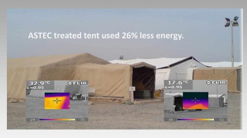
The initial test conducted over two years ago (July 2008) compared two tents located at Camp Arifjan. Although of equal size, the untreated tent had three split unit air conditioners, while the treated tent had only two units. Measurements were taken comparing the internal temperatures and a 10.8 degree Fahrenheit difference was found. Further tests were conducted and one air conditioning unit was disconnected. A 26% reduction in energy usage was realized by the use of the Astec coatings.
